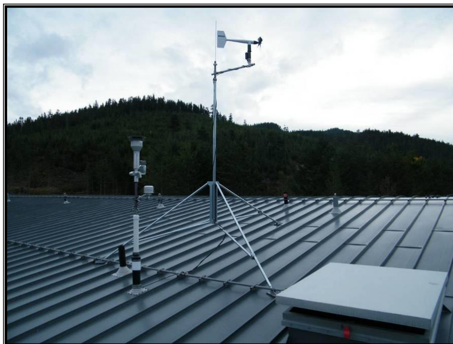
Figure 2-4 Tripod Mounted Anemometer and TEOM Inlet located on the Roof of the HPC building
