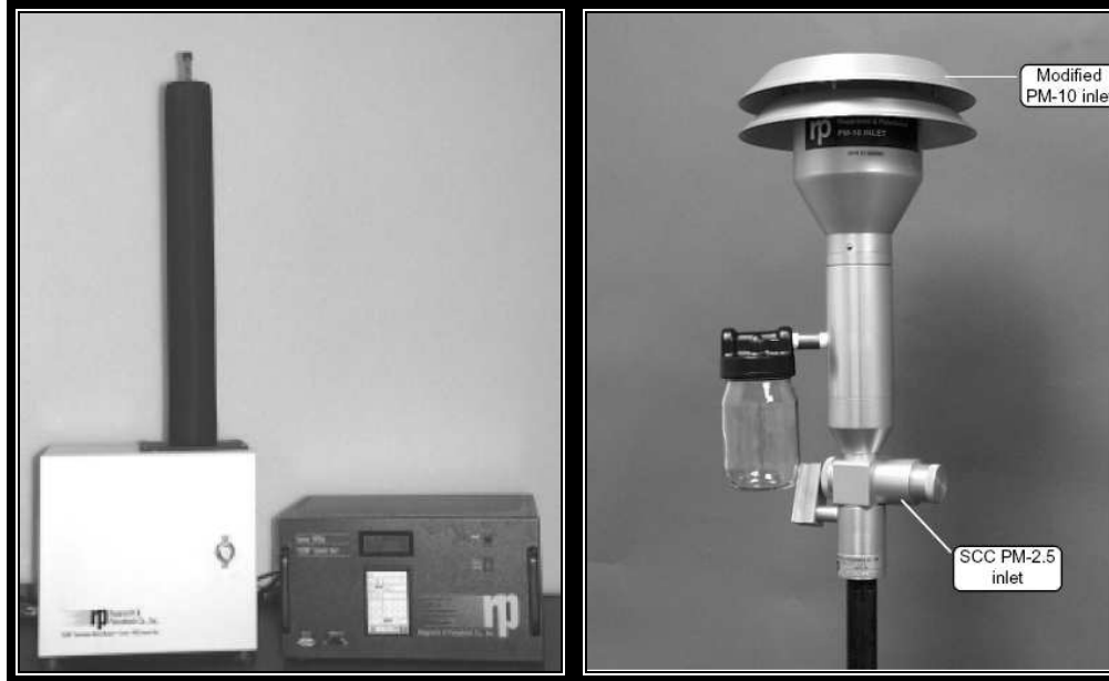
Figure 3 TEOM Sensor Unit (left), Control Unit (middle) and Inlet System (right)
