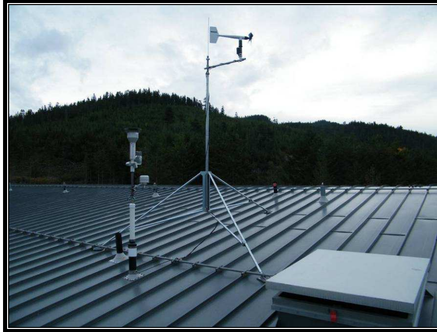
Figure 4 The Tripod Mounted Anemometer and TEOM Inlet located on the Roof of the HPC building
