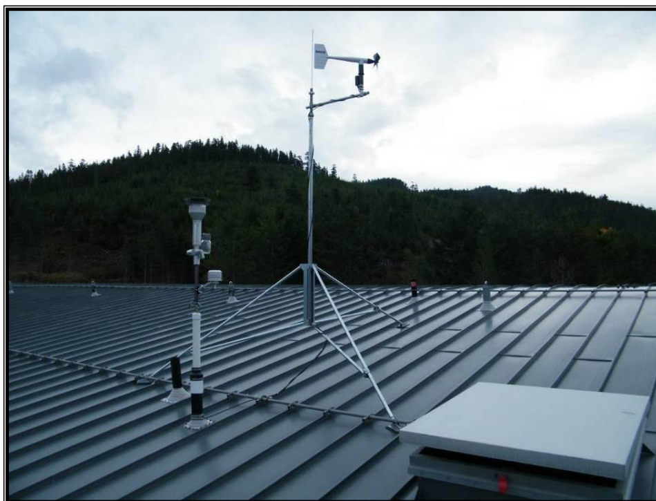
Figure 4 Tripod Mounted Anemometer and TEOM Inlet located on the Roof of the HPC building
