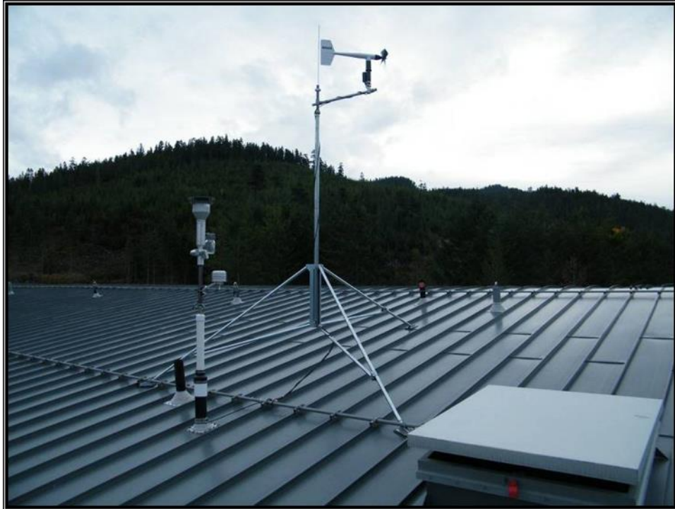
Figure 2-4 Tripod Mounted Anemometer and BAM Inlet located on the roof of the HPC Building
