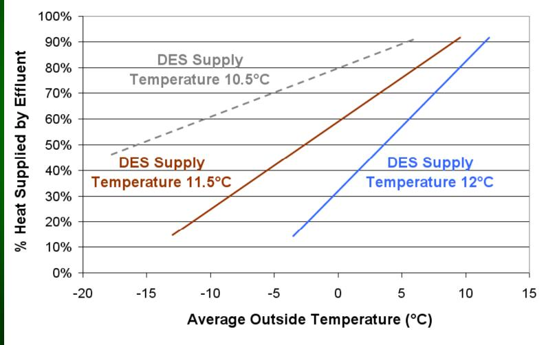
Notes - solid lines: operational results; dashed line: system design parameters.
