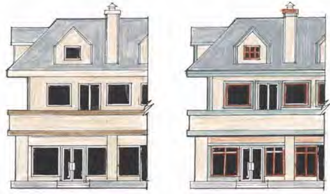
Many Whistler buildings lack trim details on the facade.
