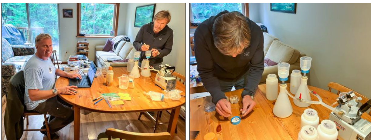
Photo 5-4. (left) Water from field replicates is filtered. (right) Once pumping is finished, the filter paper is removed and prepared in sterile packaging for shipment to the lab.
