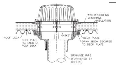
Remove existing roof drains, Install Zurn roof drains or equivalent.
