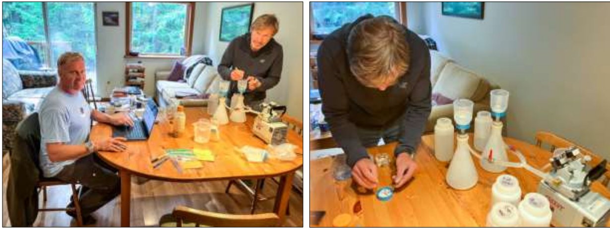
Photo 5-4. (left) Water from field replicates is filtered. (right) Once pumping is finished, the filter paper is removed and prepared in sterile packaging for shipment to the lab.
